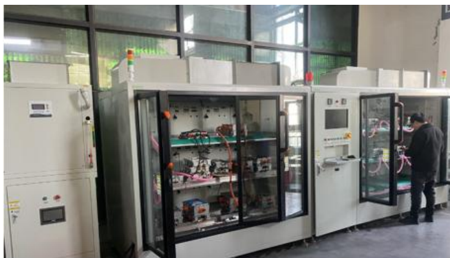
Aging load cabinet
